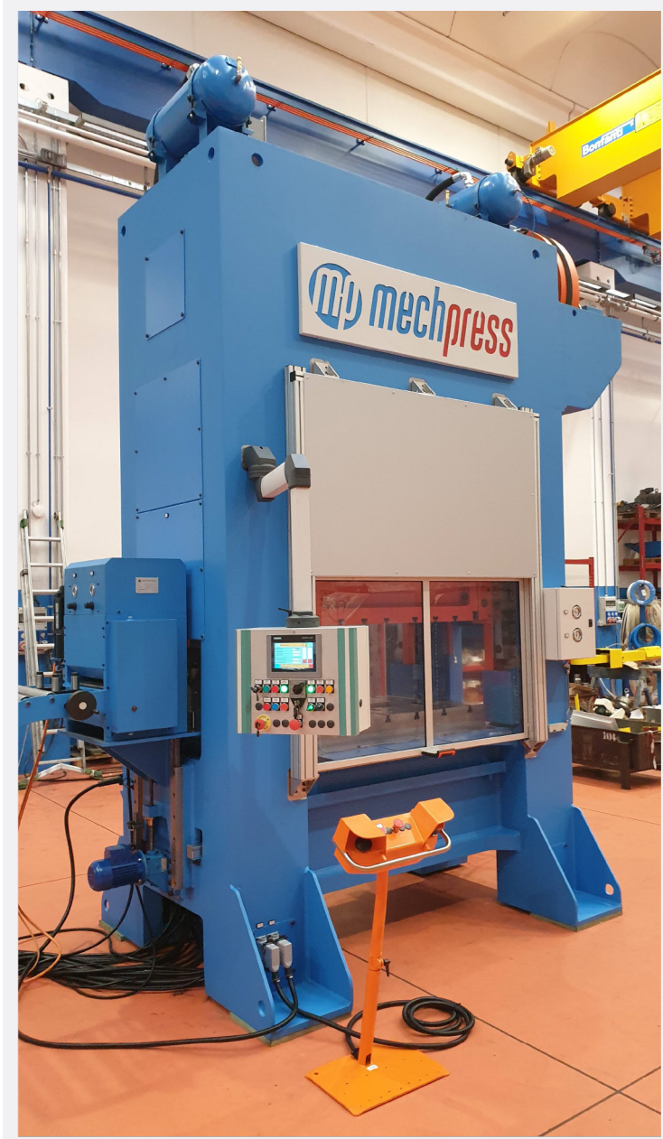
2 Connecting Rod, 160 Tons, Table 1250x400 mm
